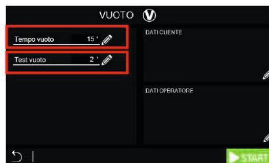
i) While the vacuum phase is running, if the SKIP button is pressed, the vacuum pump stops running and the unit starts the vacuum test.
